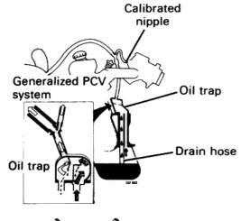
The crankcase emission controls prevent crankcase gases from being released into the atmosphere. Instead, the crankcase gases are directed to the intake manifold. Crankcase gases are removed from the crankcase by positive crankcase ventilation (PCV). Engine vacuum draws the crankcase gases out, thus allowing fresh air to be drawn in.
