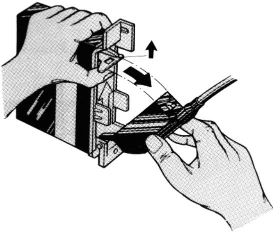
**Removing connector on Electronic Control Unit.**
