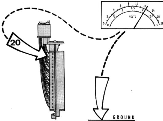
**Test voltage across terminal 20 in connector and ground. Ignition ON.**
