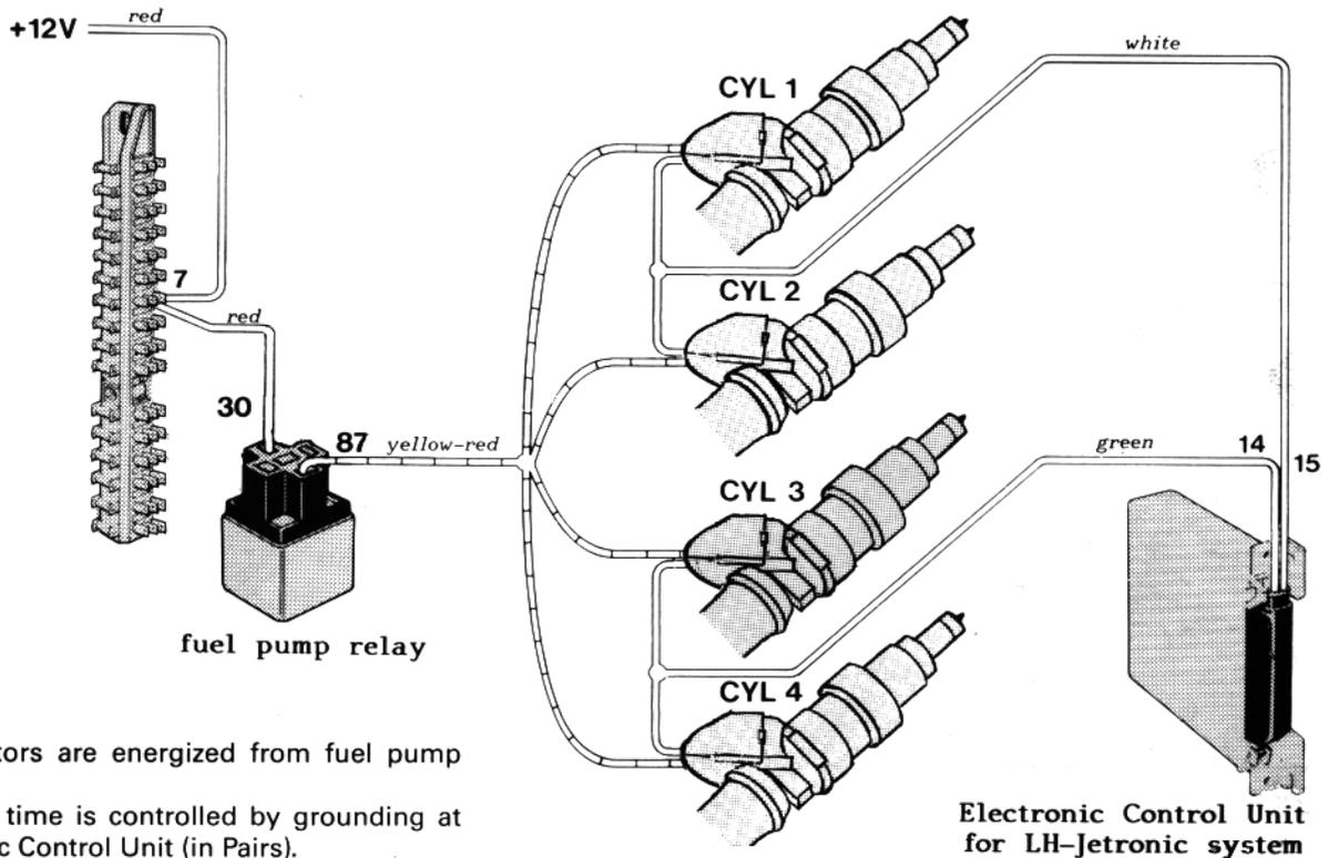
All injectors are energized from fuel pump relay.
