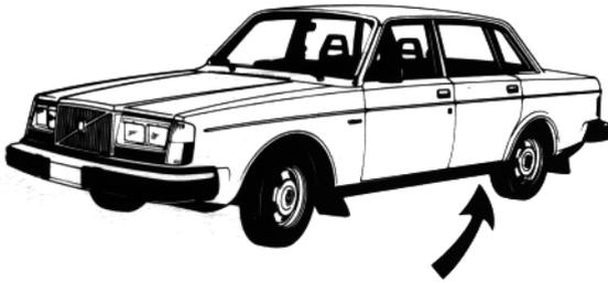
Fuel pump and fuel filter are attached to a bracket underneath the car, under left rear seat.
