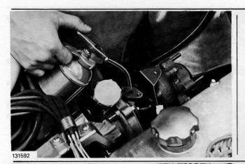
Fill turbo-compressor oil inlet with oil.
