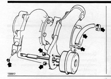
Use standard procedures to replace pressure actuator.
