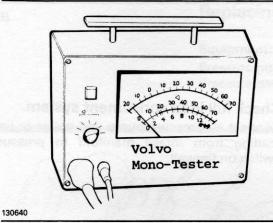
Instruments used are Volvo Mono-Tester or "Magnetic Timing Units" equipped with proper adapter.
