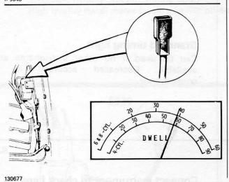
Engine running, pump air presssure until dwell meter (measuring duty cycle of lambda sond system) displays steady reading of **58.5°** (56–62° allowed). Air pressure reading at that instant should be **20.3 kPa** = 2.9 psi.
