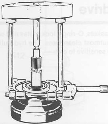
Pull off the bearing on the output shaft.
