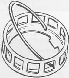
14. To assemble, install the spring in the holes in the cage.
