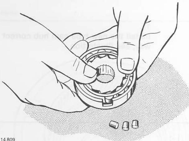
10. Rotate the one-way clutch in the ring tool so that the rollers come out, one by one.
