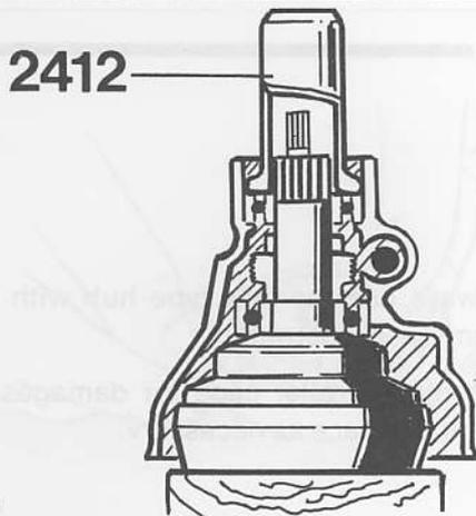
Use a piece of wood to support the output shaft.
