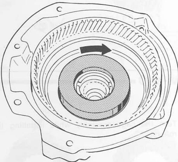
Position ring tool and one-way clutch assembly. Turn one-way clutch hub clockwise while pressing one-way clutch into position.
