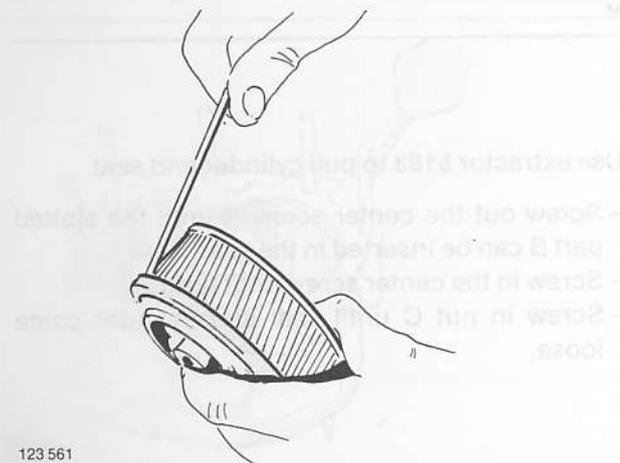
Use a screwdriver to pry loose the oil slinger.
