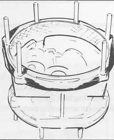
Position gasket and brake drum on front housing.
