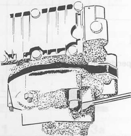
Remove the nuts holding front and rear housings
