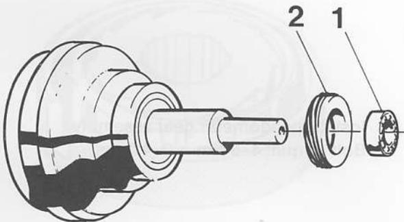
Install speedometer drive gear (2) and spacer (1) on the output shaft.
