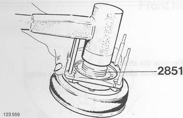
Remove the snap ring. Use drift **2851** and a plastic mallet to tap out the clutch disc.
