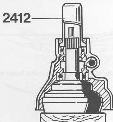
Use drift **2412** to press in oil seal in rear housing.
