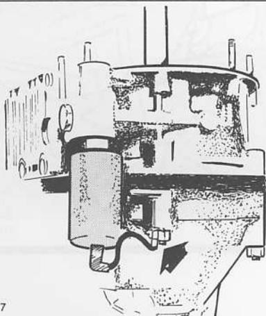
Install solenoid and ground wire.
