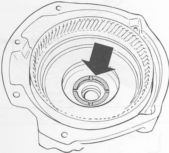
Make sure the thrust washer is properly located. If necessary, use grease to hold it in place.
