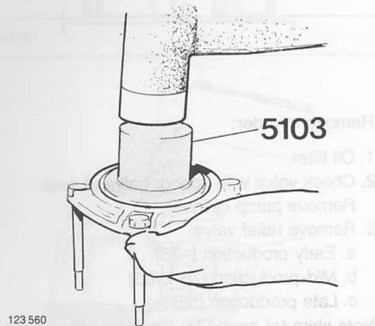
Remove the large snap ring. Use drift **5103** and a plastic mallet to tap out the bearing.
