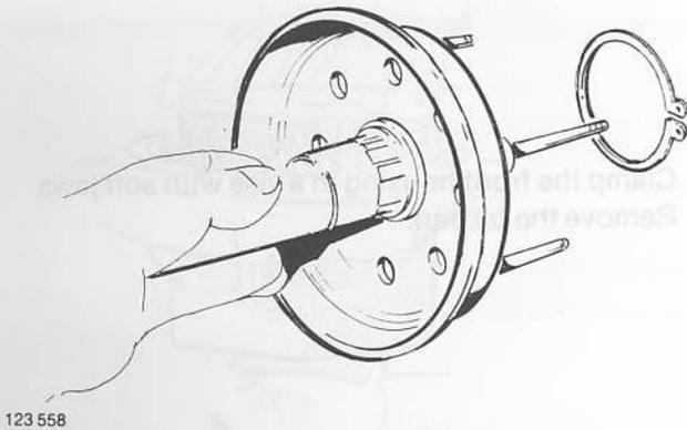
Remove the snap ring. Pull out the sun gear.
