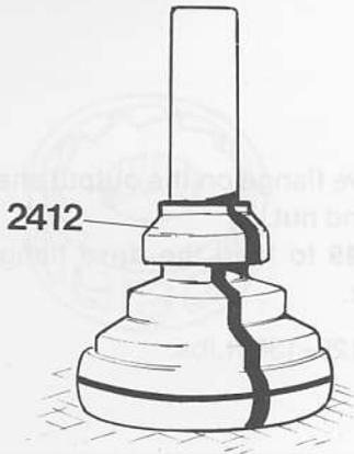
Use drift **2412** to press the bearing on the output shaft.
