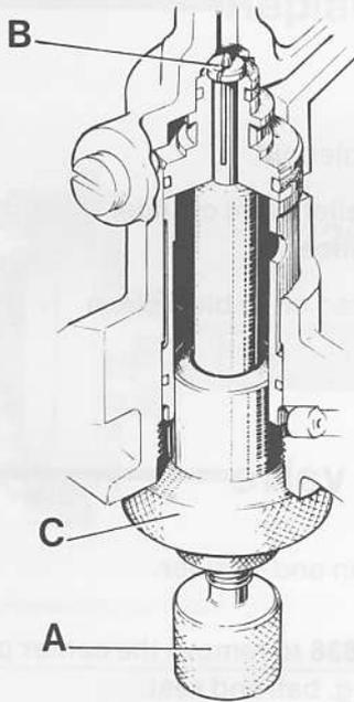
4. Use tool 5183 to pull cylinder and seat.
