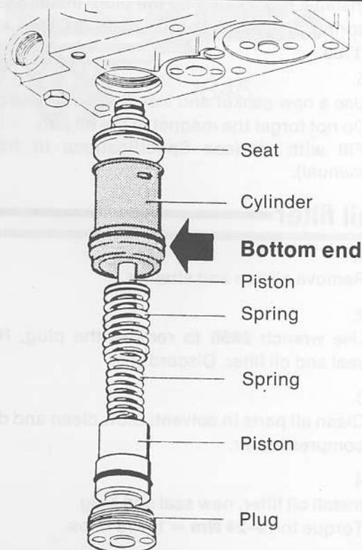
8. Position the seat in the housing. Use the cylinder to press it into correct position.
