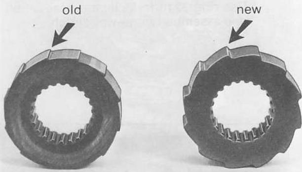
10. Disassemble and clean the one-way clutch.
