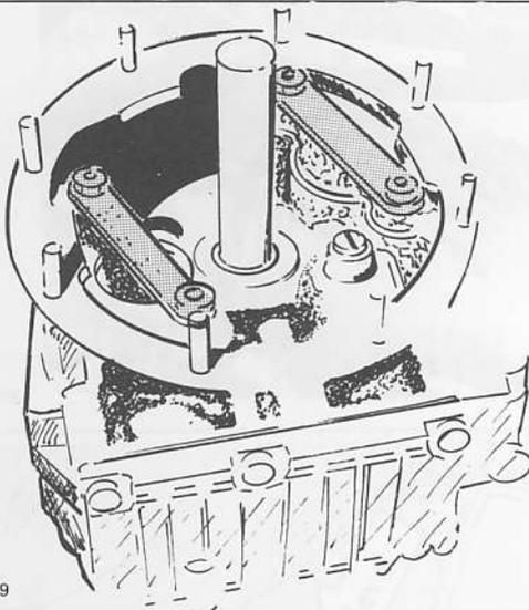
Install the bridges and tighten the nuts.
