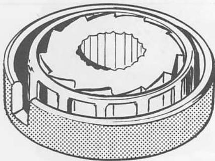
16. Install cage and hub assembly in ring tool.
