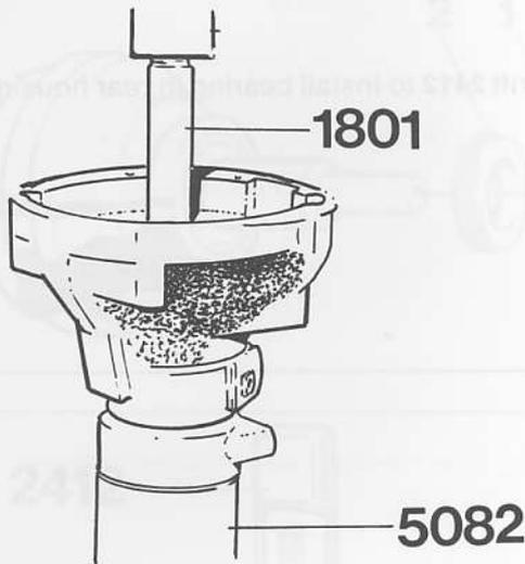
Use drift 1797 and standard handle 1801 when pressing out the bearing in the rear housing.
