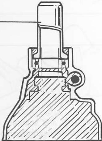
Use drift 2412 to install bearing in rear housing.
