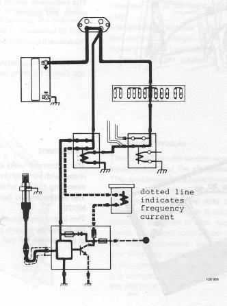
Oxygen sensor feedback system B C oxygen sensor frequency valve pump relay test instrument pick-up point main relay, oxygen sensor feedback system E electronic module D
