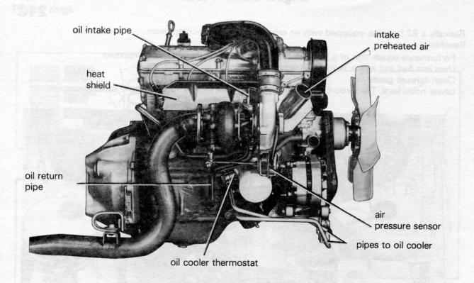
This engine is shown without catalytic converter. See "Turbo engine modifications" in this manual.
