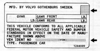
GVWR = Gross Vehicle Weight Rating GAWR = Gross Axle Weight Rating
