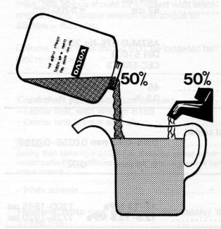
A new type coolant has been introduced for the Volvo diesel engines. It has a special chemical composition and is marked BLUE.
