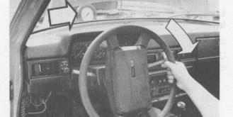
Check pump pressure at right side end position.
