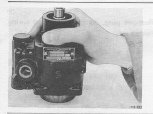
Remove rotor and cam ring.
