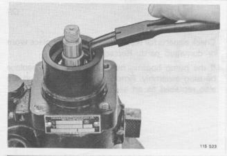
Remove ball bearing retaining ring.
