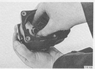
**Push out thrust ring.**Also push out cam ring, if remaining.
