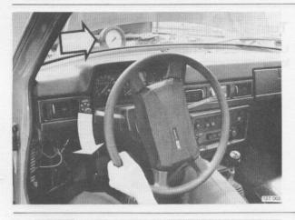
Check pump pressure at left side end position.
