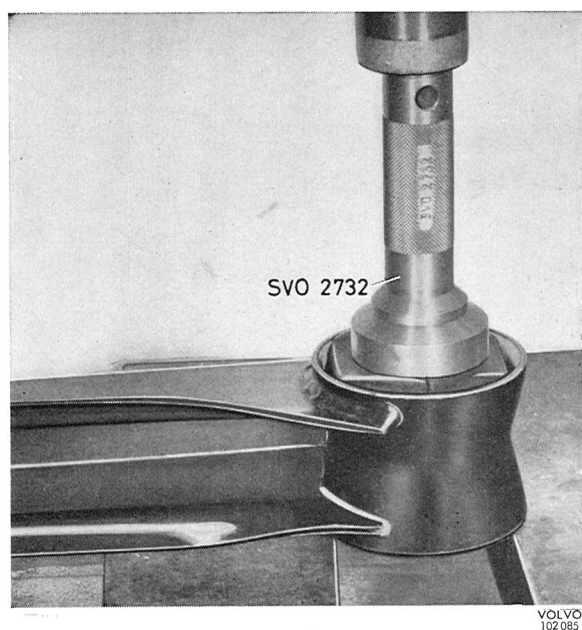
Fig. 7-11. Removal (installation I), front bushing, trailing arm
