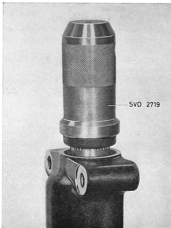
Fig. 6-61. Fitting sealing ring, pitman arm shaft
