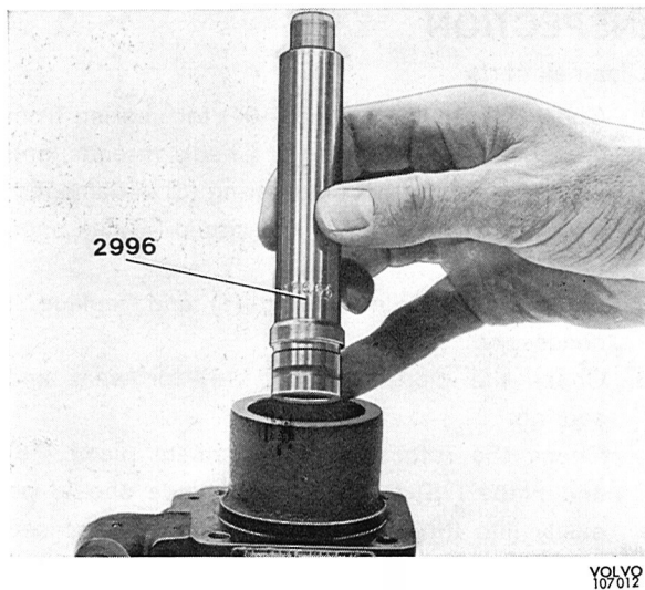
Fig. 6-107. Installing needle bearing
