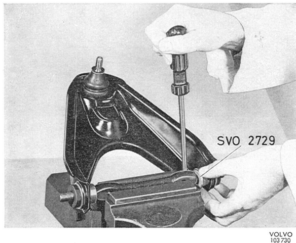
Fig. 6-33. Removing control arm shaft. 1. Removal of tool 2729
