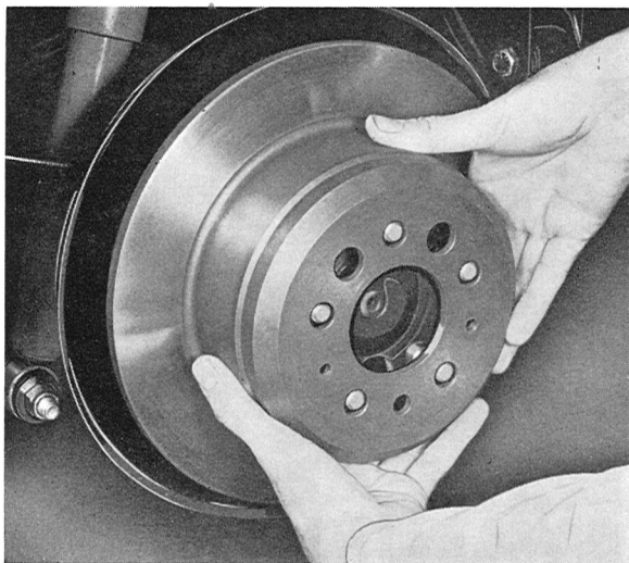
Fig. 5-81. Removing brake drum
