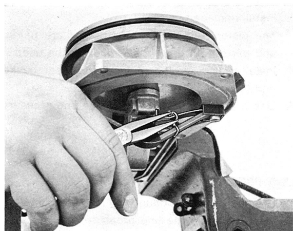
Fig. 2-188. Adjustment of air flow sensor plate level
