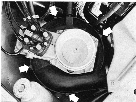
Fig. 2-190. Removal of air cleaner upper part
