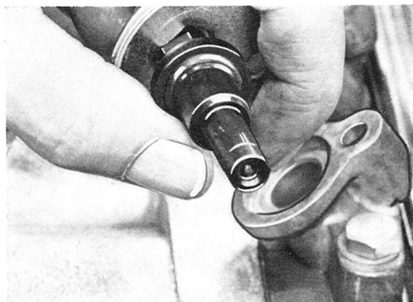
Fig. 1-35. Checking the fuel distributor for interior leaks.
