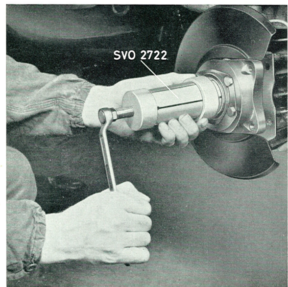
Fig. 6-16. Removing the inner bearing
