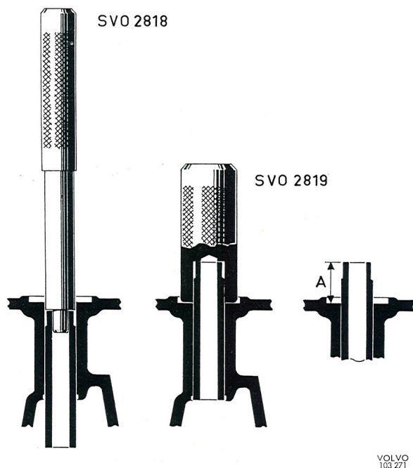
Fig. 2-28. Replacing the valve guides A=17.5 mm (0.689")
