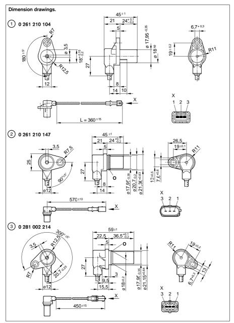
The sensor generates one output pulse per tooth. The pulse amplitude is a function of the air gap, together with the toothed ring's rotational speed, the shape of its teeth, and the materials used in its manufacture. Not only the output-signal amplitude increases with speed, but also its frequency. This means that a minimum rotational speed is required for reliable evaluation of even the smallest voltages.
