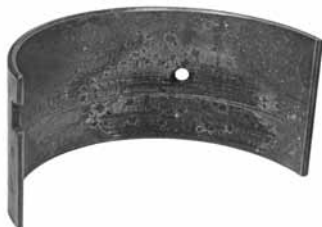
FOREIGN PARTICLES IN LINING ..... PAGE 3
