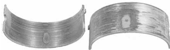
FOREIGN PARTICLES ON BEARING BACK ..... PAGE 4
