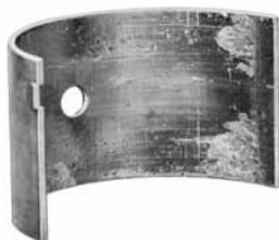
EXCESSIVE CRUSH ..... PAGE 7
