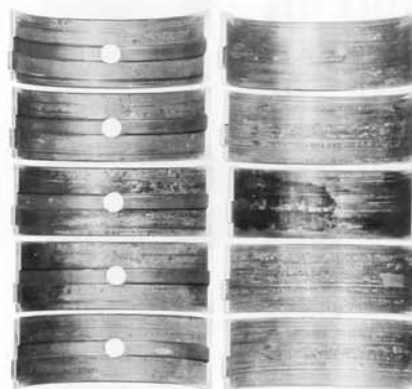
BENT CRANKSHAFT ..... PAGE 12
