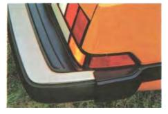
At speeds up to 10 miles per hour against a fixed barrier, the protruding front bumper will flex seven inches to absorb the impact and to protect the car body from damage. The rear bumper flexes three-and-one-half inches against a movable barrier at the same speed.
