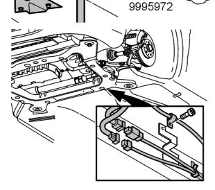
Remove the bracket for the heated oxygen sensor (HO2S) from its mounting (6 cylinder engines only). Lower the rear edge of the sub-frame approximately 90 mm. Ensure that the steering gear screws are released from the sub-frame. Remove the mobile jack.
