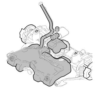
Position the cabling in the rubber grommet so that the yellow tape marking is on the inside.
