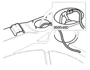
Undo venting hose <u>999 5480-2</u>. Screw the valve cap back in place.
