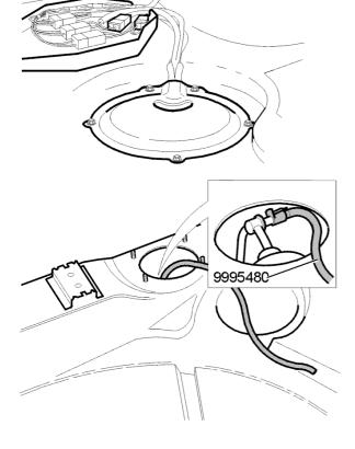
Unscrew the valve cap on the fuel line. Connect the venting hose <u>999 5480-2</u>.
