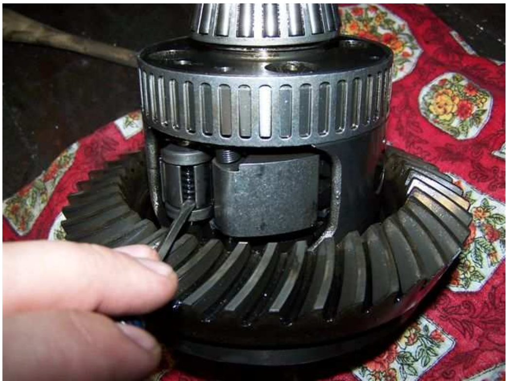
At low speeds (below 25 MPH) the governor pawl sits in this position, held by a torsion spring:
