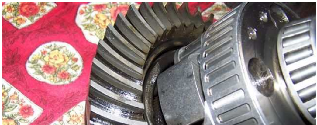
At low speeds (below 25 MPH) the governor pawl sits in this position, held by a torsion spring:
