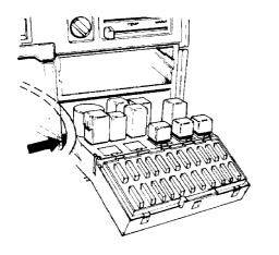
Remove fog lamp relay, position F
