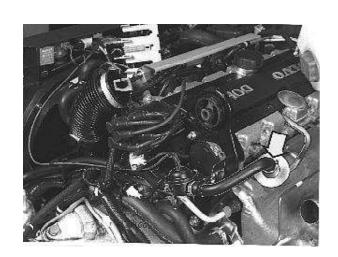
Disconnect the rubber hose to the relief valve and start the engine.
