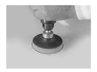
Spread 3M Finess-It 9631 over the surface thinly. Polish the surface with an oscillating machine for 12–15 seconds, though not more than 15 because the "pad" gets too hot. Finish polishing with lighter strokes.
