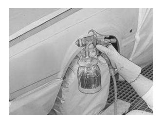
Allow the primer coat to air dry (approximately 20–30 minutes, 20°C (68°F)). Spray filler should not be directly applied to etching primer.
