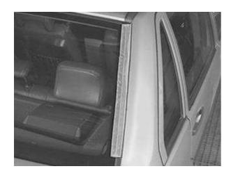
often sufficient to fully mask off the repair area.
