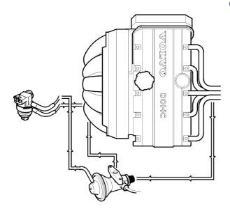
A proportion of the exhaust gases is recirculated to the intake manifold to reduce emissions of nitrogen oxides (NOx) in the exhaust gases. NOx gases form at the high temperatures which occur in engine combustion at high loads.
