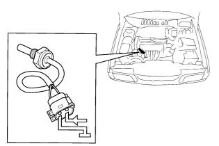
The ECT sensor on the thermostat casing provides the control module with information on the ECT. The ECT sensor has a temperature–sensitive resistor with a NTC. The control module sends a nominal (no–load) 5 V voltage to one of the sensor connections, while the other is connected to ground. Depending on the ECT and hence the sensor's resistance, the voltage from the control module varies. The voltage is high when the engine is cold and low when it is hot.
