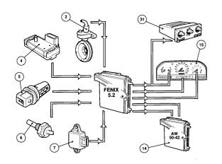
The control module supplies some other systems in the car with data it takes from the sensors.
