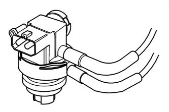
The EGR controller regulates the vacuum pressure to the EGR valve from the outlet on the top of the EGR controller. The vacuum from the intake manifold is supplied to the underside of the EGR controller. The controller stabilises the vacuum from the intake manifold and converts the electrical signal from the control unit to a vacuum signal for controlling the EGR valve.
