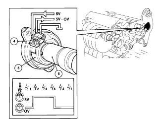
The CMP sensor has a Hall generator which helps the control module decide the different cylinders' working cycle.
