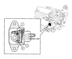
The TP switch is mounted on the throttle casing, and tells the control module how wide the throttle is open. This information is used to determine acceleration and engine load.
