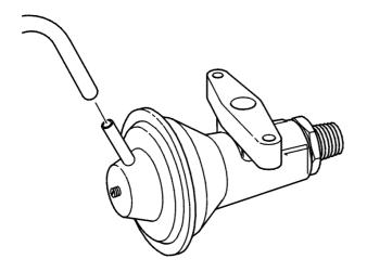
The EGR valve controls the flow of gas from the exhaust manifold to the inlet manifold. The valve is controlled by the vacuum in the line connected to the EGR controller. The EGR valve is located underneath the inlet manifold.
