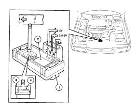
5 V voltage. Depending on the pressure in the intake pipe, the membrane bends to a varying extent and its resistance alters. The PCB notes this change, and adjusts and amplifies the signal so that the output signal from the pressure sensor varies between 0.5 and 5 V, depending on the pressure.
