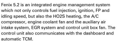
The unique feature of Fenix 5.2 is that the injectors operate individually for each cylinder ('sequential injection'). The advantage of this is that fuel is injected at the optimum time for combustion and the injectors can be controlled individually.
