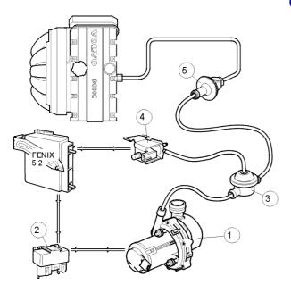
The auxiliary air system is designed to minimize hydrocarbon and carbon dioxide emissions when starting from cold and to heat the catalyser up faster. By adding fresh air to the exhaust ports when starting the engine from cold, the air pump helps burn off uncombusted hydrocarbons. This enables the system to increase the injection time and retard the timing, increasing the exhaust gas temperature and activating the catalyser faster.
