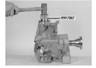
Ensure that the tool goes towards the bevel gear housing.
