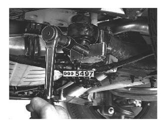
Install press tool 999 5497 on the trailing arm
