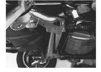
Bend down the trailing arm mounting from the bodywork locating pin on right-hand side
