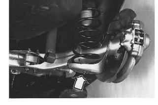
Install the shock absorber. Tighten the nut a few turns
