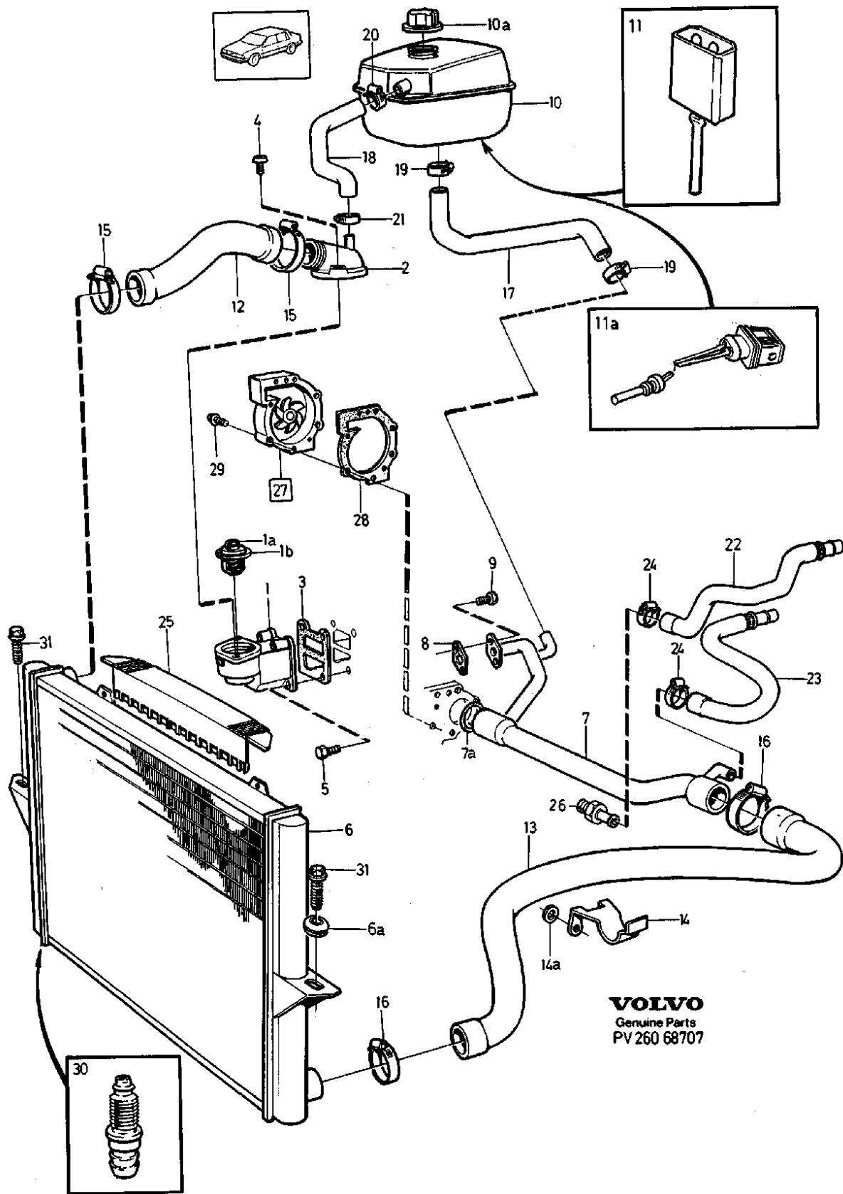
**Cooling system. 5CYL. 4VALVE TURBO**
