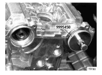
Keep the central screw of the belt tensioner fixed and turn the eccentric of the belt tensioner anti-clockwise until the tensioner dial passes the marked position and reaches its end position.
