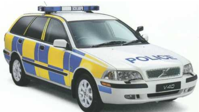
VOLVO S40 AND V40 POLICE CAR Front-wheel drive. Alternative engines: four-cylinder 136-bhp petrol engine, turbocharged 165-bhp or 200-bhp petrol engines or a 115-bhp direct-injection turbodiesel. Five-speed manual gearbox or five-speed adaptive automatic transmission. Chassis with DSA anti-skid system and automatic height control.
