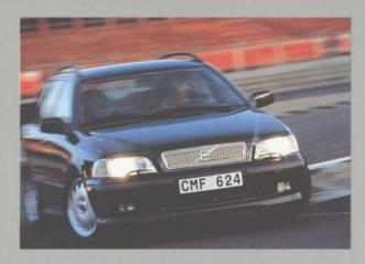
The T4 chassis is designed to ensure excellent handling. It has fast rack and pinion power assisted steering and independent suspension all round (in sport and comfort settings), to produce a car which will handle twisty roads with composure and efficiency. All that get up and go is matched by equally impressive stopping capacity. The T4 benefits from the latest in anti-lock braking technology - Electronic Brake Distribution (EBD).
