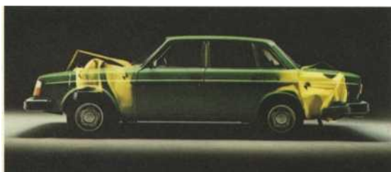
Front and rear ends have energy-absorbing crumple zones.
