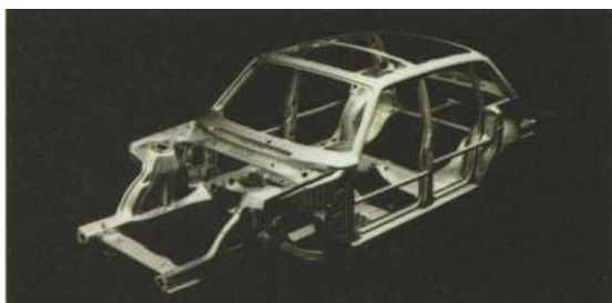
closed section profiles form a reliable safety cage.
